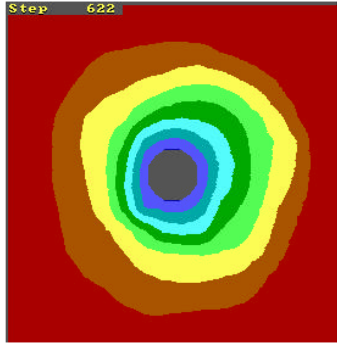
Figure 8. Sample pore pressure distribution in model after several iterations.
