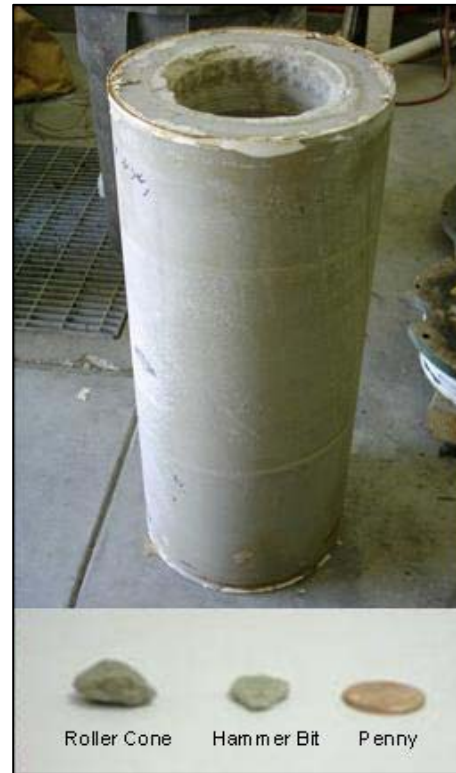
Fig. 6. One drilled rock sample and collected cuttings from a roller cone drilling test and a hammer drilling test.
